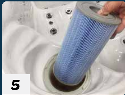
5 Insert the filter and place it over the circular holding piece so it sits tight.
