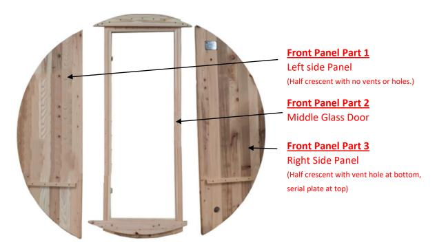
Before securing the front panels together, consideration must be made for the wiring of the Lamp / Sauna light. The included lamp does not come with wiring or a switch, these must be provided and installed via an electrician. A wire channel is provided in the 'Front Panel Part 3' as shown below.
